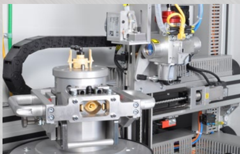
Detail of process head installed on motorized YZ unit.
